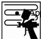
Apply 2 single coats, allowing for a 8-10 minutes of flash off time.
