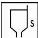
Spray Viscosity – 18 – 22 Secs in B4 Cup at 30°C
